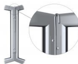
HARNESS ATTACHES TO CORNER BRACKET ON PERFEX SKYFRAMES
